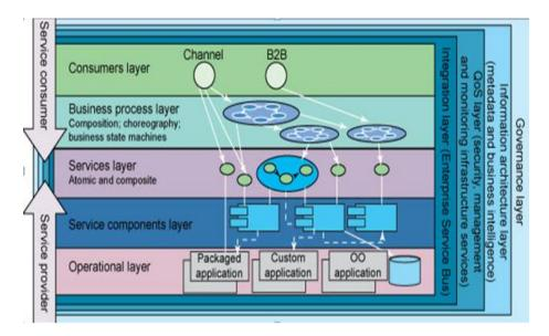
Figure 2. Layers of SOA reference architecture [5].
